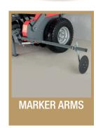
Tracer arms moving with hydraulic piston support.
