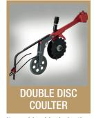
It provides ideal planting thanks to its offset positioned, serrated and flat discs and cast pressure wheel.
